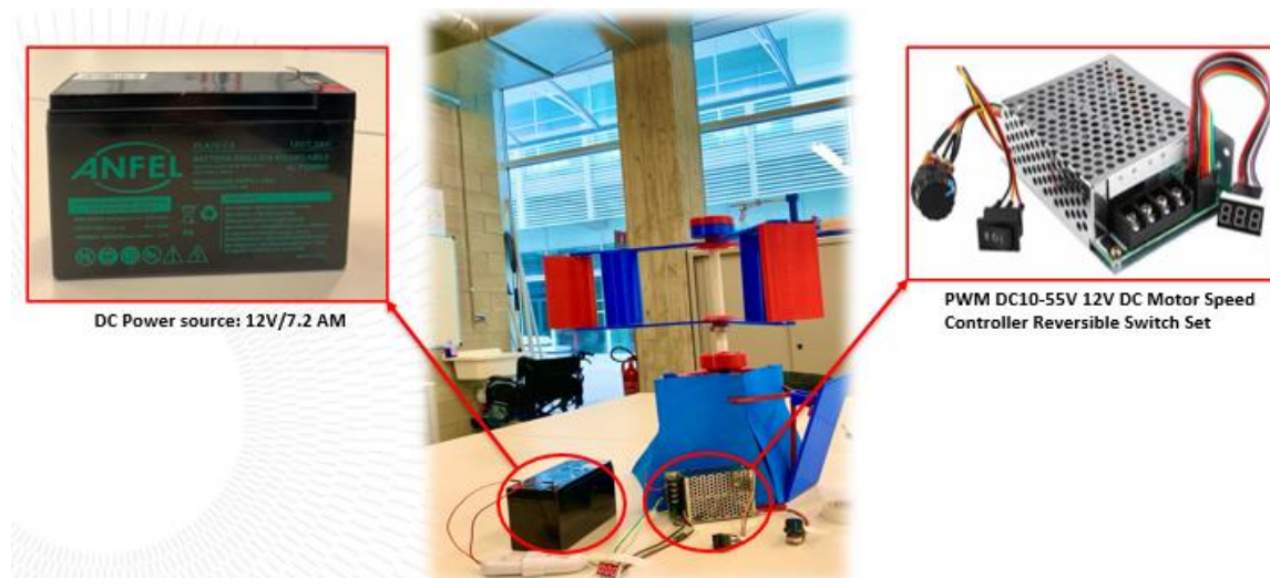
Figure 9: Power source on the left and the speed controller on the right.
